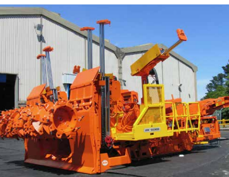
The 12CM30 miner bolter has a wide installed base in longwall entry development applications in Australia, with an increasing presence in the Eurasian market. Over 15 years of continuous improvements and developments are incorporated in the latest models.
