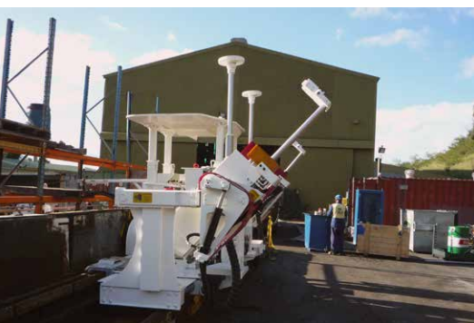
Roofbolts can be placed on the faceside or angled into the longwall face in a variety of different positions and different bolt centres.
